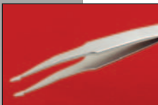
SM106 4 3/4" 120 mm For positioning all SOT packages horizontally. With flat base tips (4 mm long)
